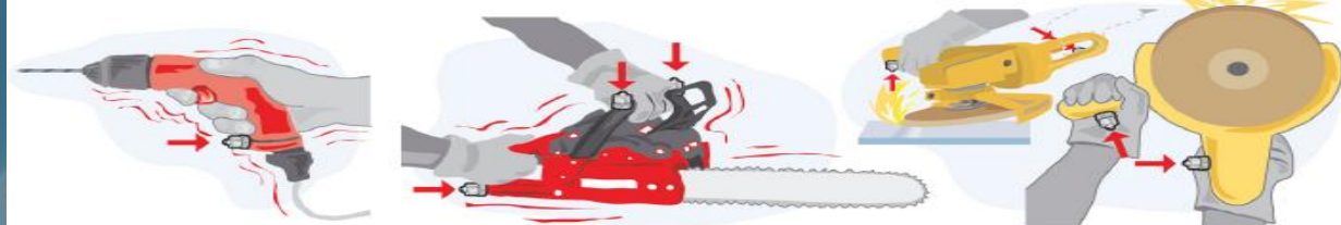
Example of accelerometer mounting positions.
